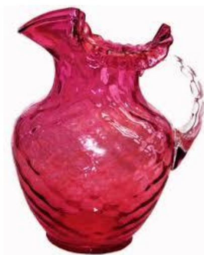
Fig. 4.2.2 Glass carafe in which gold nanoparticles are dispersed (this glass is known as ruby glass).
