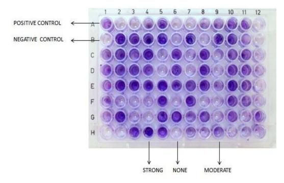
Fig 2: Tissue culture plate method for detection of biofilm formation.
