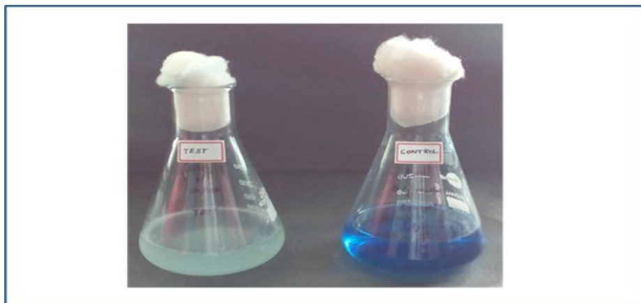
Figure. 3: Degradation of diesel by heavy metal resistant isolate.
