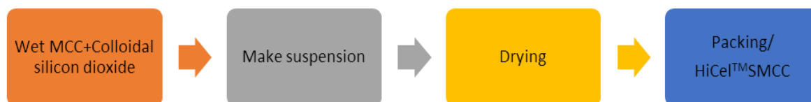
Fig2. Manufacturing process of HiCel™SMCC.
