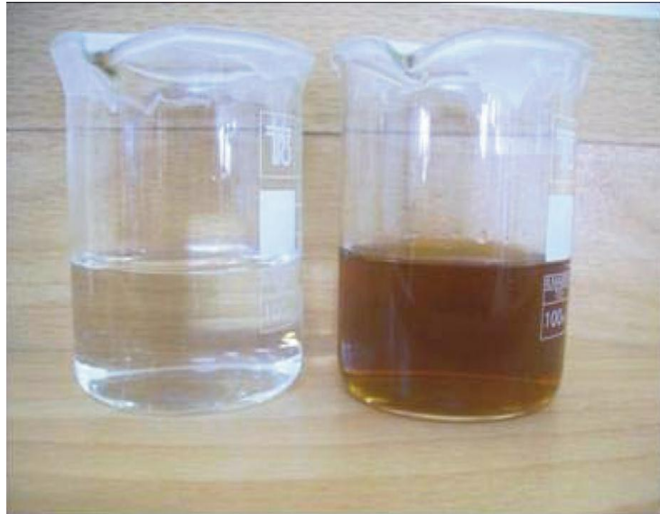
Figure 1: A solution of silver nitrate (3 mM) before (left) and after (right) addition of plant extract solutions.
