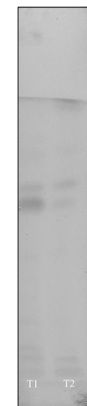
Figure 4: High-performance thin-layer chromatography of optimized Kashaya Rasa Dominant Zone selection (after spray with vanillin H 2 SO 4 ), T1 - Spot of Kulattha , T2 - Spot of Kanchanara solvent system-chloroform:MeOH (9.5:0.5)
